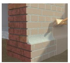
a level 15 cm below the bottom edge of the foundation footing up to 30 cm above ground level. Allow the mortar to cure properly. This procedure should be omitted for dry masonry.compounds BOLIX – waterproofing in existing buildings
